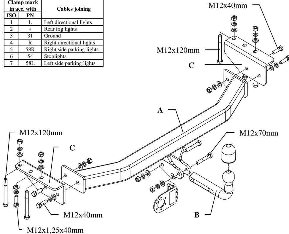
This towbar is designed to assembly in following car: **MITSUBISHI PAJERO SPORT, 5 doors, (K90)** produced since 07.1996 till 2008, catalogue no. **Z29** and is prepared to tow trailers max total weight **2800 kg** and max vertical load **115 kg**.
