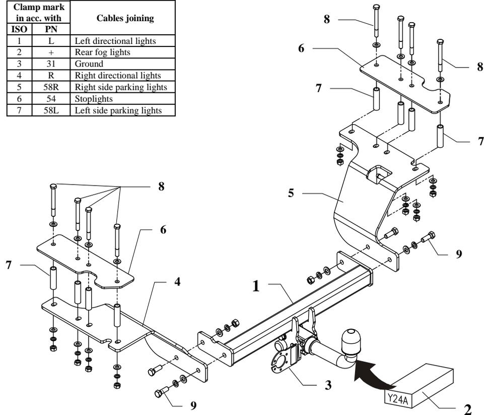
This towbar is designed to assembly in following cars: **HONDA CR-V, 5 doors** produced since 04.2002 till 01.2007, catalogue number **Y24A** and is prepared to tow trailers max total weight **1690 kg** and max vertical mass **100 kg**.
