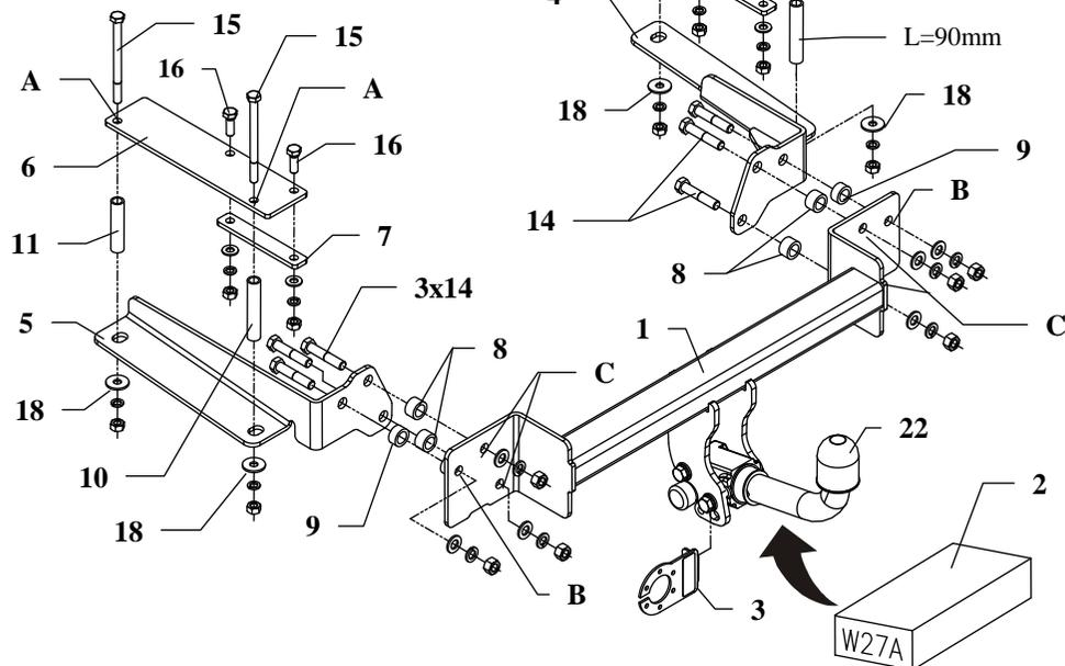
This towing hitch is designed to assembly in following car: **SUZUKI SX4 4 DOORS**, produced since 11.2007 till 09.2013, catalogue number **W27A** and is prepared to tow trailers max total weight **1200 kg** and max vertical mass **50 kg**.
