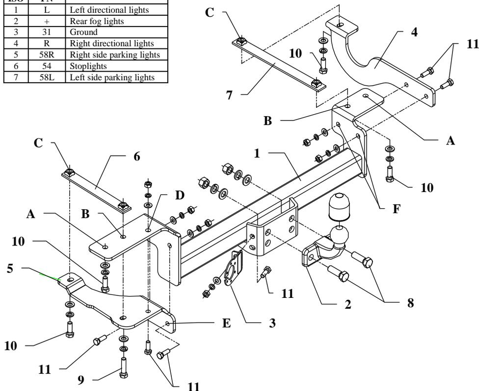
This towing hitch is designed to assembly in following cars:
