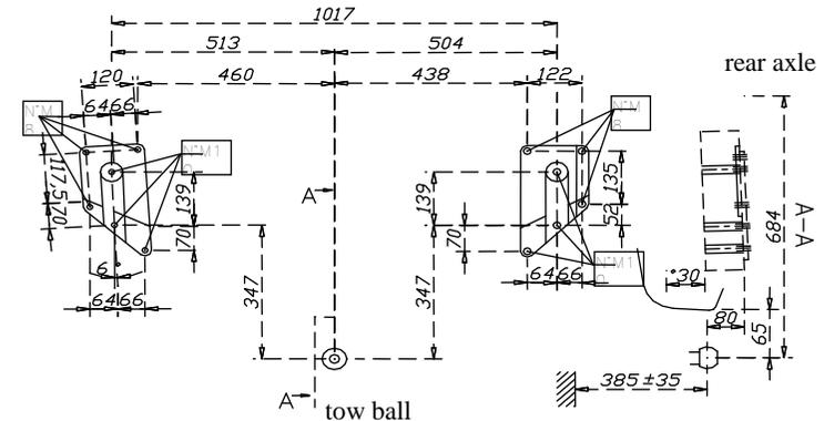
4. On drilled holes put fish-plates (pos. 7 and 8). Holes pos. A on drilled holes.
