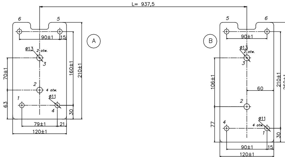
Figure 2. Fish-plates placement
