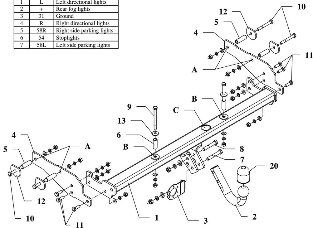
This towing hitch is designed to assembly in following car: **CITROEN C15, delivery van**, produced since 1985 till 2007, catalogue no. **P06** and is prepared to tow trailers max total weight **900 kg** and max vertical load **45 kg**.
