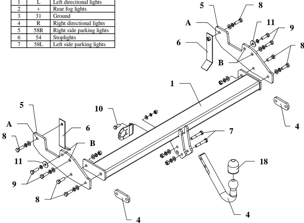
This towbar is designed to assembly in following cars: **TOYOTA HILUX 4WD with double cabin**, produced since 10.2005 till 10.2010, catalogue number **O64** and is prepared to tow trailers max total weight up to **2500 kg** and max vertical mass **100 kg**.
