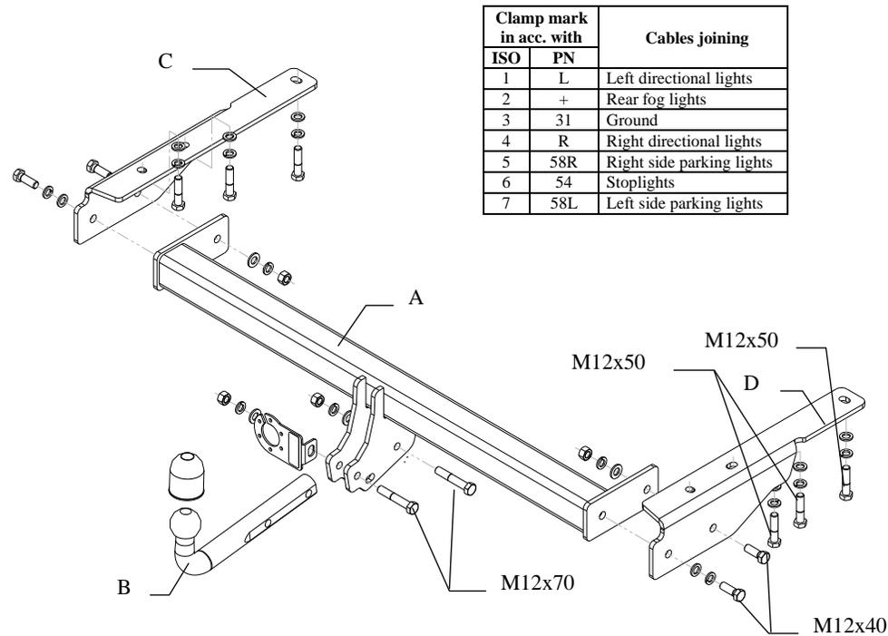
This towbar is designed to assembly in following cars:
