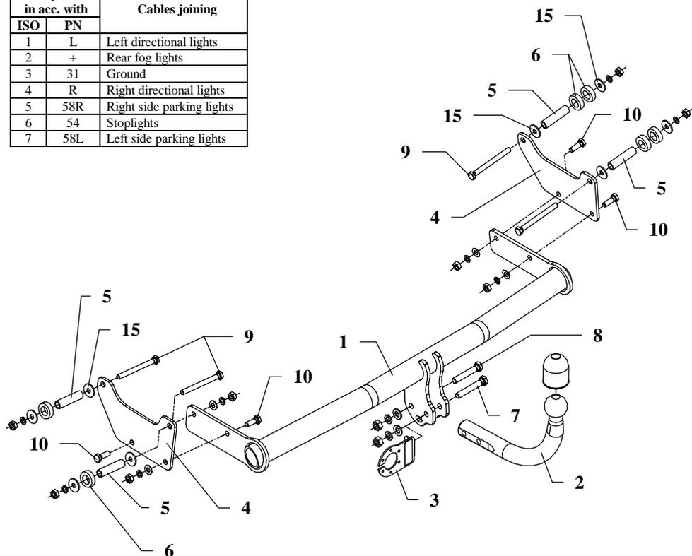
This towing hitch is designed to assembly in following cars: **RENAULT GRAND MODUS**, produced since 2008, catalogue no. **G59** and is prepared to tow trailers max total weight **1200 kg** and max vertical mass **75 kg**.
