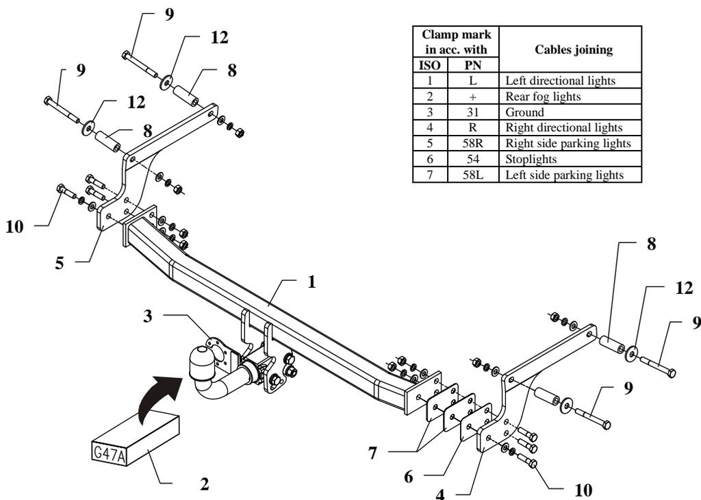
This towbar is designed to assembly in following car: **DACIA LOGAN, 4 doors**, produced since 09.2004 till 12.2012, catalogue number **G47A** and is prepared to tow trailers max total weight **1100 kg** and max vertical load **75 kg**.
