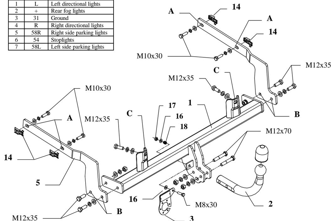
This towbar is designed to assembly in following cars: **PEUGEOT 406 D8, D9 ESTATE**, produced since 1996 till 02.1999 and since 03.1999 till 2004, catalogue no. **F08** and is prepared to tow trailers max total weight **1700 kg** and max vertical load **80 kg**.
